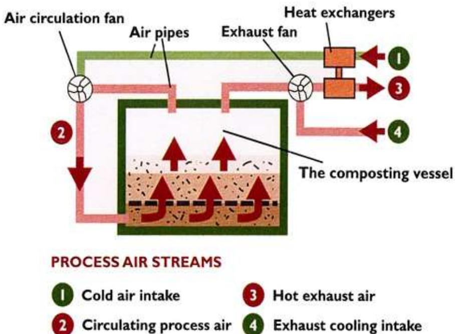
Figure 2. Schematic diagram of in-vessel process control system.
