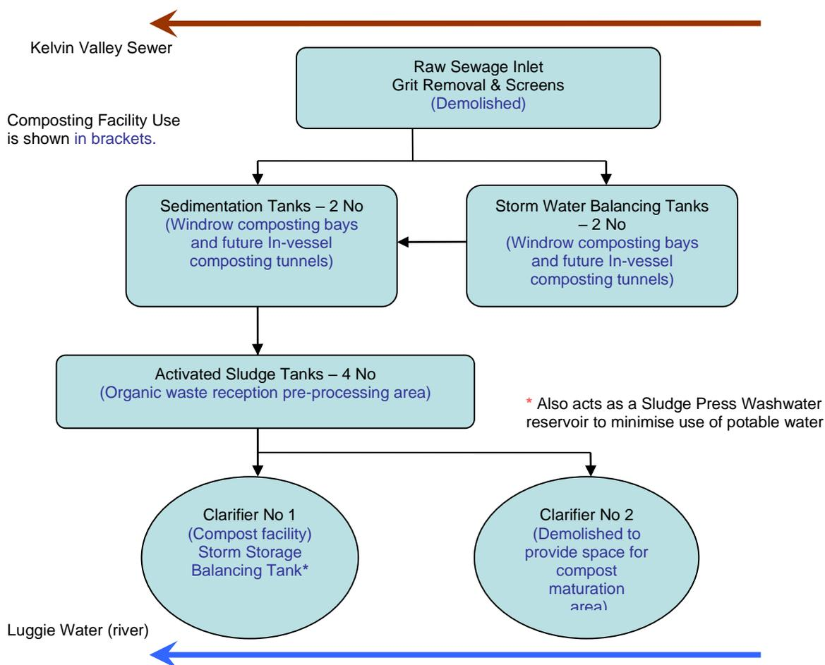
Figure 1. Schematic diagram of the Deerdykes Activated Sludge Sewage Works, with uses after conversion.
