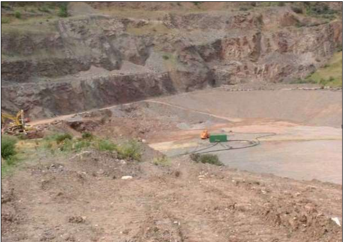
View of the quarry sump; the source of the contaminated groundwater
